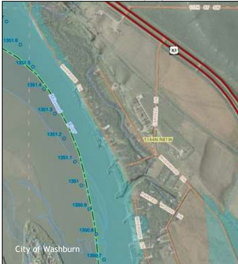
Figure 5.2-4 100 Year Flood – south of Washburn Source: FEMA
